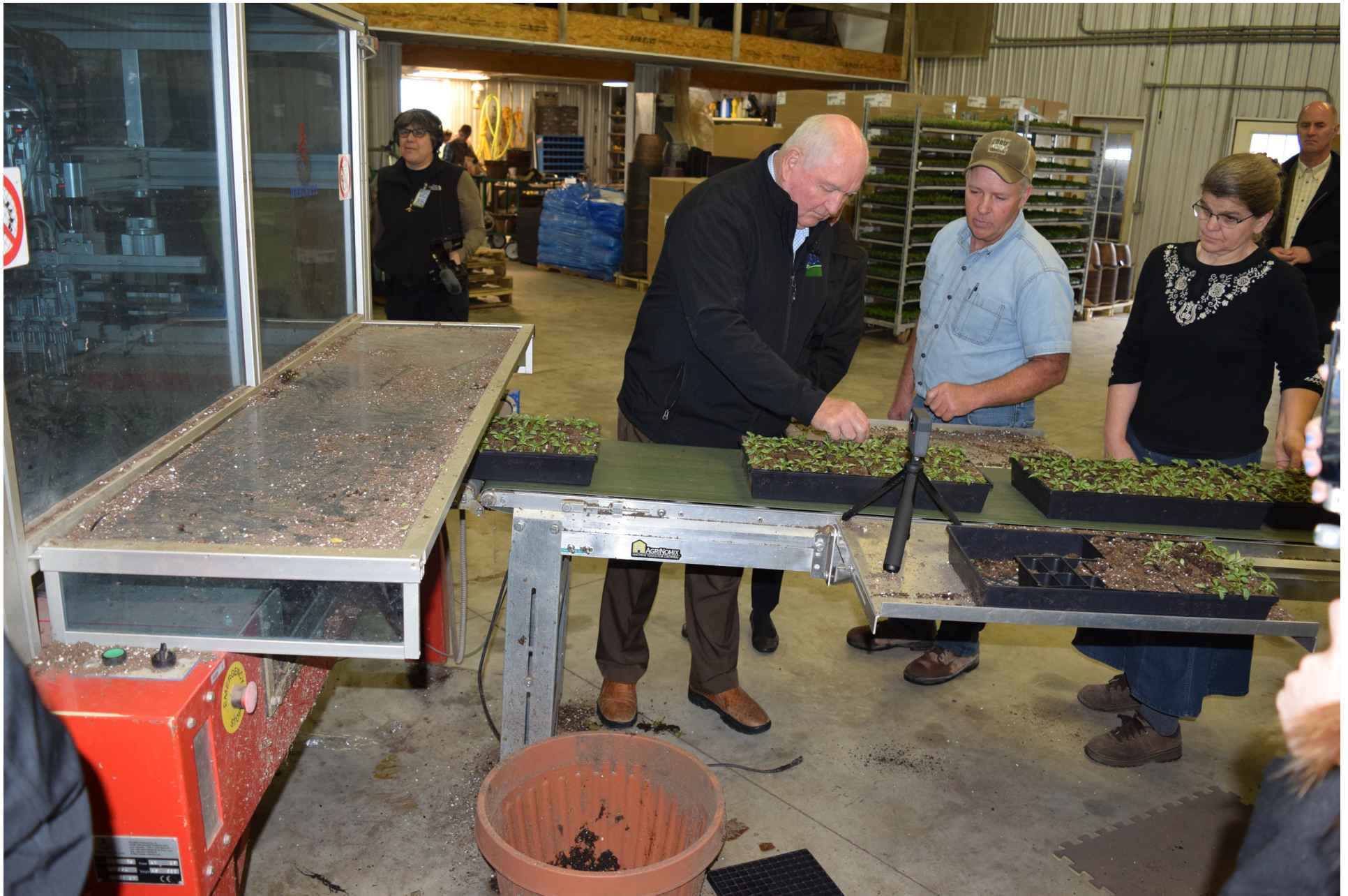
A machine that transplants seedling into flats, formerly a time-consuming job.
